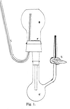
actually in the thermostat. Accordingly, the following filtration apparatus, a modification of the previous one,<sup>8</sup> was used. Its construction is shown in the diagram.
