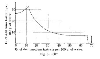
No reference to the hydration of lithium tartrate could be found in the literature, and it became advisable to determine the transition temperature of lithium tartrate dihydrate to anhydrous lithium tartrate. The dilatometric method and the solubility method were employed. By the former method the transition temperature resulted as 21.52°. The solubility figures are given in Table II.
